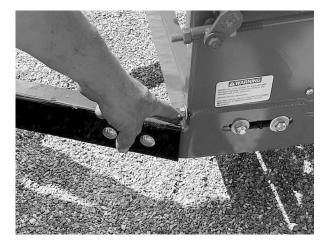
**Floor Apron Chain -** Periodically check the floor apron chain tension by pulling up on the center cross member of the floor apron.
