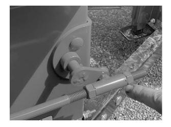
In order to adjust the chain control arm, use a <sup>3</sup>/<sub>4</sub>" wrench to loosen the nuts on either side of the slide tee, (located on the front of the control rod). Move the control rod to the front or rear as needed, and re-tighten the nuts. The adjustment is complete when the control arm lifts the chain from all of the teeth in the drive gear. You may have to repeat this adjustment several times in order to achieve the proper setting.
