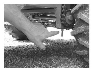
**Beater Chain -** In order to adjust the beater chain tension, loosen the nut which holds the chaintension sprocket, (5/8'' nut). Loosen or tighten the jacking nut as needed, (3/8'' nut) to adjust the chain tension. After the adjustment is set, retighten the chain tension nut.
